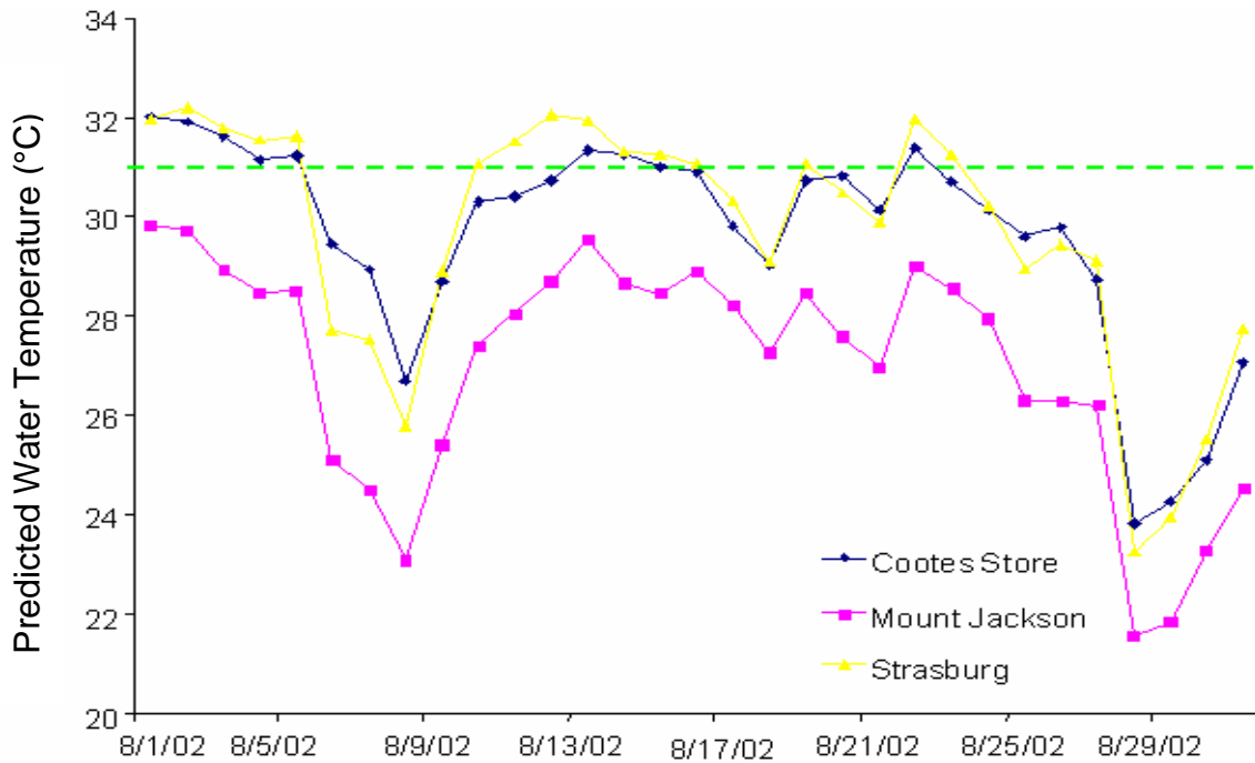
Figure 85. SNTEMP maximum daily water temperature predictions for August 2002 at the North Fork Shenandoah River gauging stations: Cootes Store, Mount Jackson, and Strasburg (sites 1, 15, and 29). The green dashed line marks the Virginia water quality standard of 31°C (State Water Control Board 2003).
